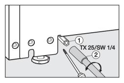
If necessary, also align the two rear adjusting devices ① using a socket wrench ②.
